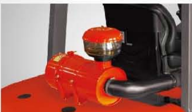
Pre-cleaner engine air intake
